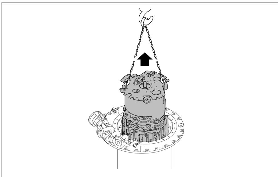
Figure 57: Retirer le corps insérable
