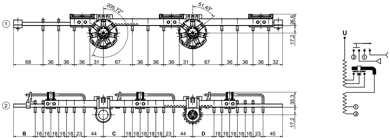
**N.B.** Maximum impulse voltage between adjacent contacts of series/parallel connection BIL= 100 kV.
