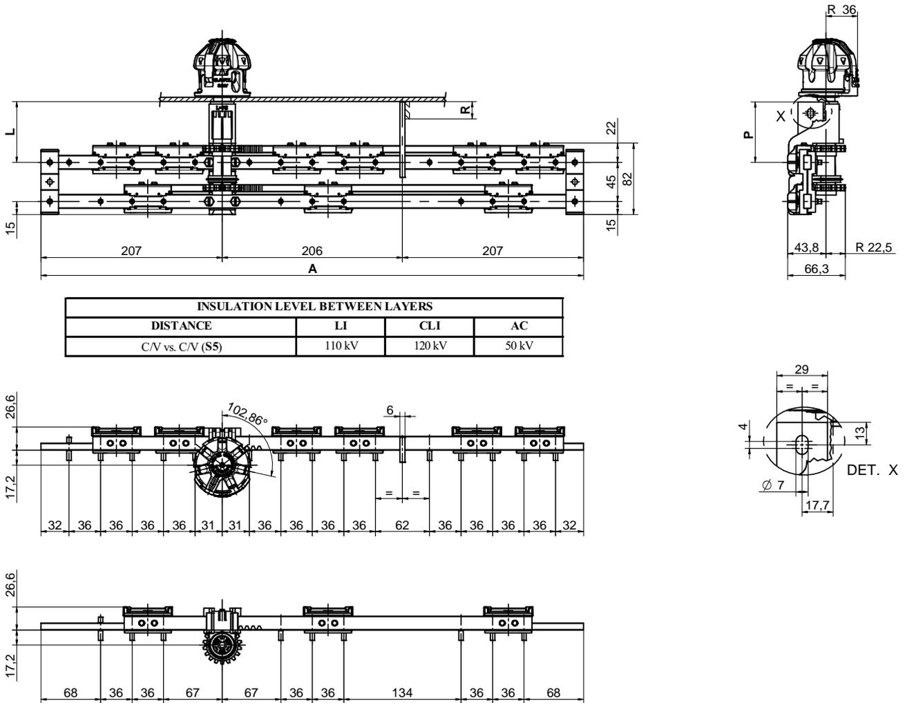
N.B. Maximum impulse voltage between adjacent contacts of change voltage connection BIL= 100 kV.
