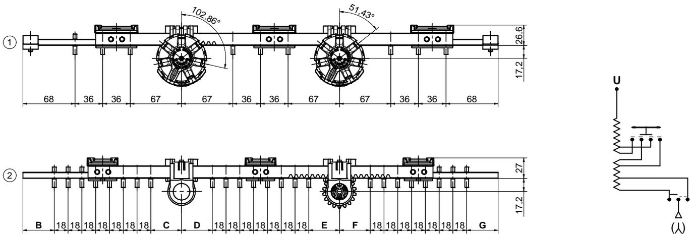
**N.B.** Maximum impulse voltage between adjacent contacts of series/parallel connection BIL= 100 kV.
