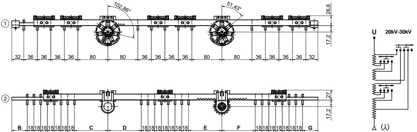
**N.B.** Maximum impulse voltage between adjacent contacts of series/parallel connection BIL= 100 kV.
