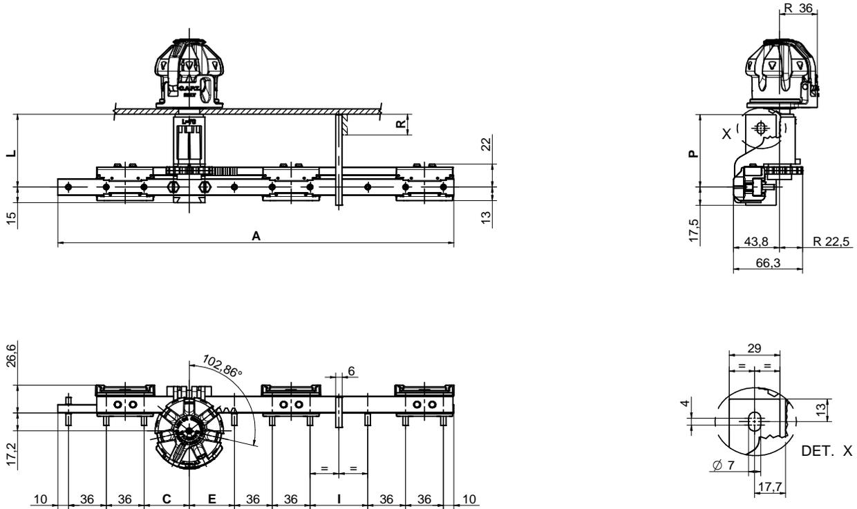
N.B. Maximum impulse voltage between adjacent contacts of change voltage connection BIL= 100 kV.
