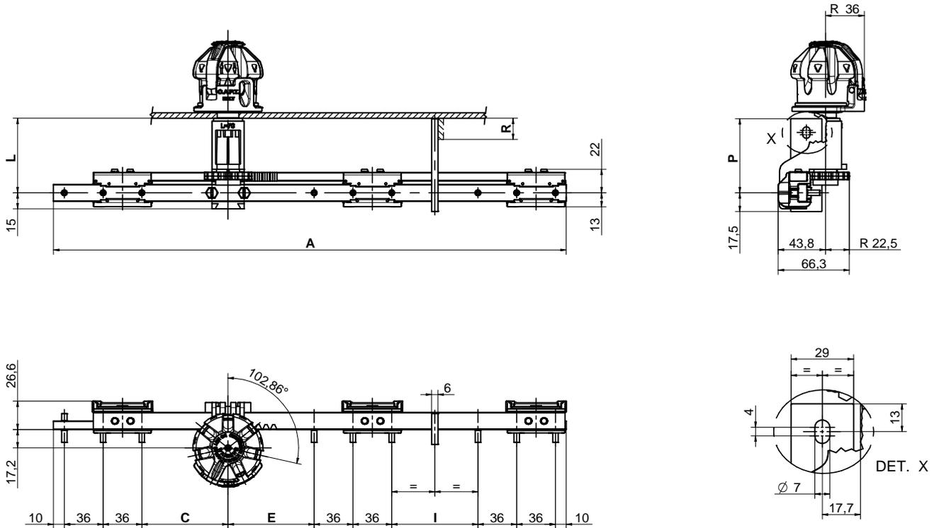
N.B. Maximum impulse voltage between adjacent contacts of change voltage connection BIL= 100 kV.
